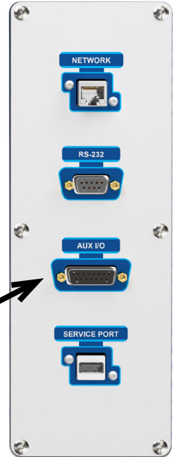
Figure 14 - Digital feedthrough panel
