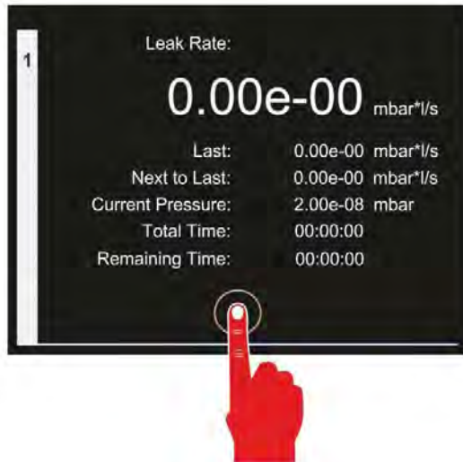
Figure 31 – Starting Leak Test
