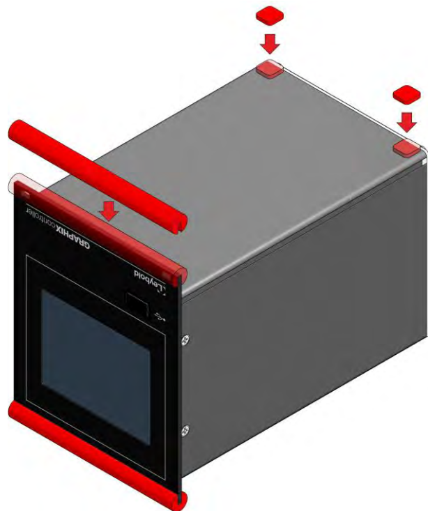
Figure 6 – Preparing the bottom side of the instrument for utilisation as a benchtop unit
