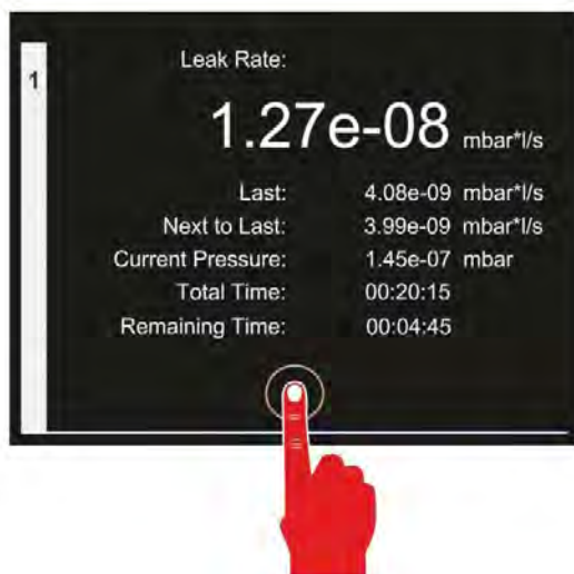
Figure 32 – Stopping Leak Test
